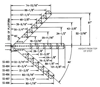
\* (Aluminum model numbers shown. For steel, replace "SS-40#" with "SS-20#")
