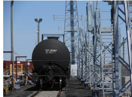
The client wanted the ability to load multiple, compatible products from each loading spot. A product selector arm, spring-balanced and articulated for ease of use, was designed so that operators could easily move between different product feed lines, depending on what the customer had ordered to be loaded into the rail car.
