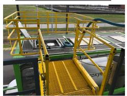
The client had a need for a new loading station that would allow for safe employee access to overseas shipping containers. Due to the nature of the chemical being loaded, the system had to be able to withstand a harsh and corrosive environment. It was important that the chemical not be diluted with water during inclement weather. Therefore, a custom integrated canopy was required. Benko Products specializes in engineering our equipment to meet our client's specific needs.
